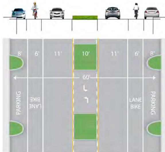
Option 2: Reduce travel lanes and add median islands interspersed with turn lanes; add interspersed landscaped curb extensions to inset parking
