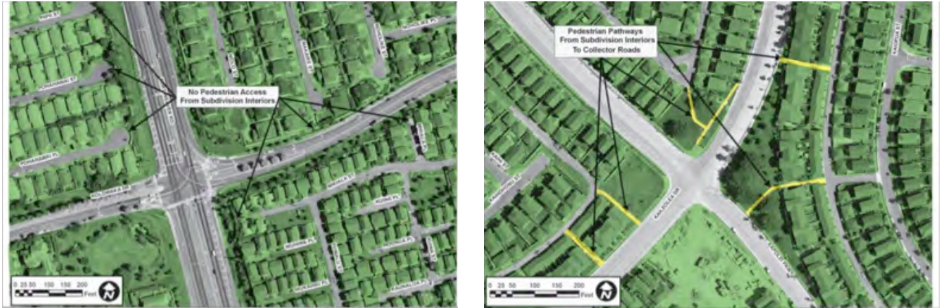
Above, left: Cul-de-sac break up connections. Above, right: Pedestrian networks can be re-established by opening noise walls and connecting new sidewalks (Credit: PB Americas, EWA Connection Study, May 2009)
