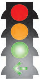
Protected-permissive left-turn signal
