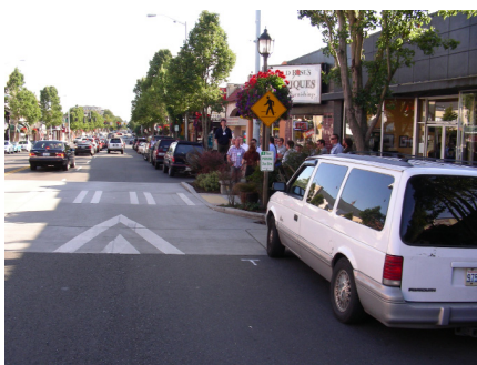
Periodic traffic calming measure: Raised crosswalk in Seattle, WA (Credit: Ryan Snyder)
