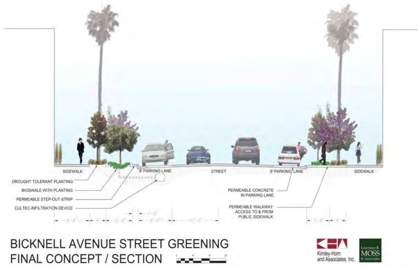
Parkway incorporating streetwater tools: Bicknell Avenue, Santa Monica, CA (Credit: Neil Shapiro)
